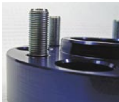
(Left) Spidertrax wheel spacers are made of 6061T6 anodized aluminum and machined to exacting tolerances to fit specific vehicles. XJ, KJ, ZJ, CJs, YJs and TJs are available in 1.25-inch thickness. JK, WK and Commanders are 1-3/8 to 1.5 inches thick, depending on the application needed. (Right) Spidertrax wheel studs come pre-installed and include the necessary lug nuts and thread-locking compound.
